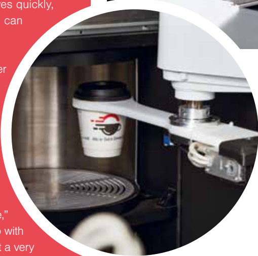
Robotic arms take the brewed coffee and move it to the delivery window for pickup.
