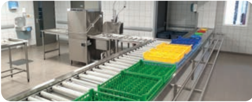
Pass-through machine with automatic hood-lift system
