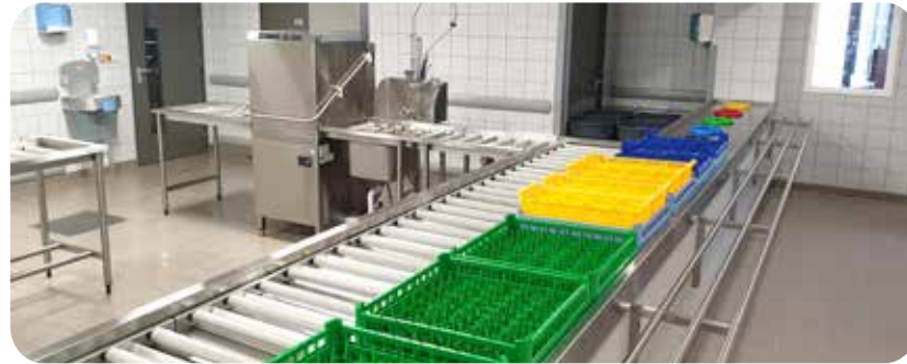
Pass-through machine with automatic hood-lift system
